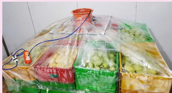
Pilot adopting of forced air-cooling system after VHT treatment to reduce waiting time by 4-5 hours at Hoang Phat
